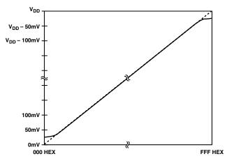
Figure 19. Endpoint Nonlinearities Due to Amplifier Saturation
